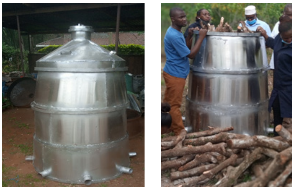
Fig.24: The newly procured portable metal kiln (left) and the kiln being loaded with wood at Mtwapa Energy Centre (right)
